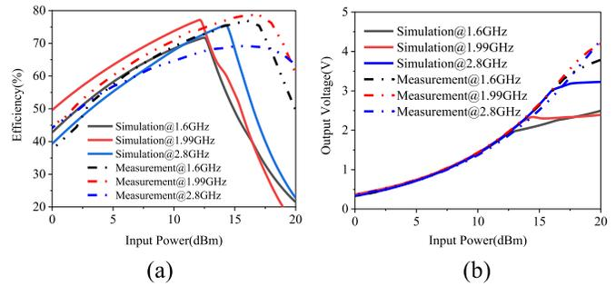
Fig. 11. (a) Conversion efficiency (b) Output Voltage from 0 dBm to 20 dBm at 1.6 GHz, 1.99 GHz, and 2.8 GHz.
