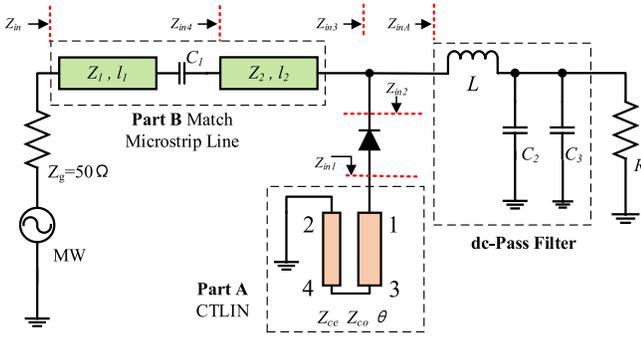
Fig. 1. Proposed rectifier with a wide bandwidth range.
