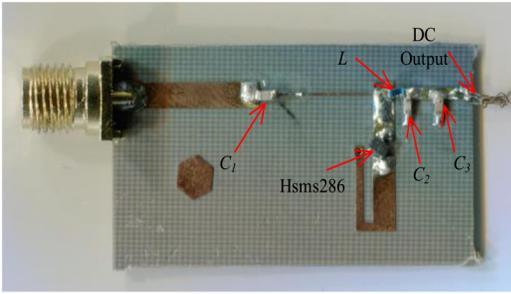
Fig. 7. A photograph of the fabricated rectifier.
