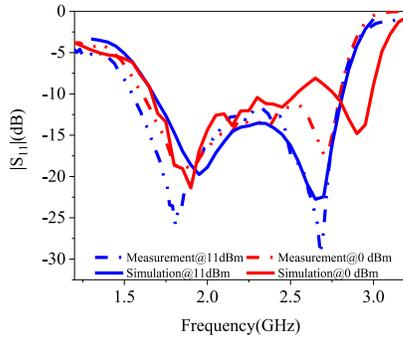
Fig. 8. The reflection coefficient  $|S_{11}|$  versus frequency at the input power of 0 dBm and 11 dBm.
