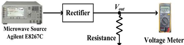
Fig. 9. Diagram of the measurement system.
