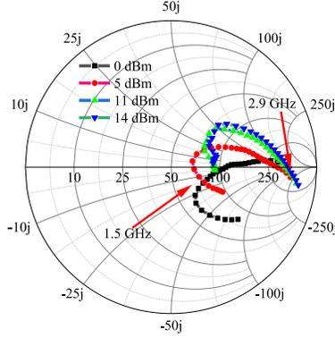
Fig. 4.  $Z_{in2}$  over 1.5-2.9 GHz at various input power levels.
