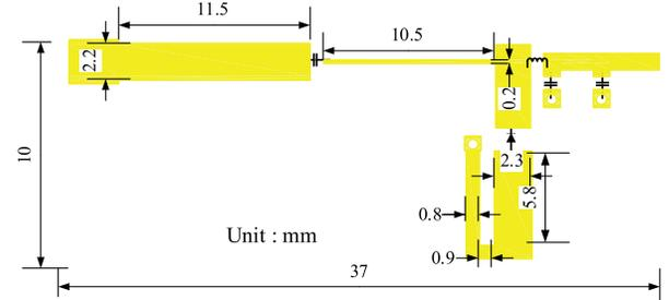
Fig. 6. Layout of the proposed broadband rectifier.
